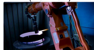
Chamber Components (Aluminum, thermal spraying)
