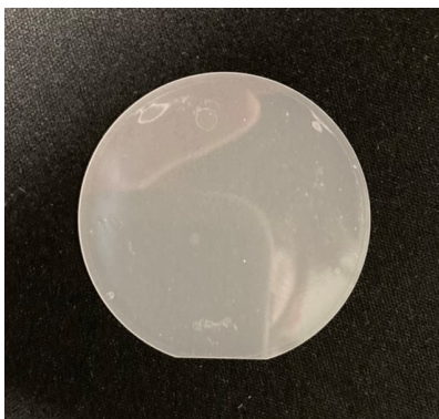
Next-generation power semiconductor wafer prototype (2-inch wafer)
