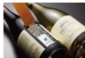
An example of wine bottles with sensor tags attached to them
