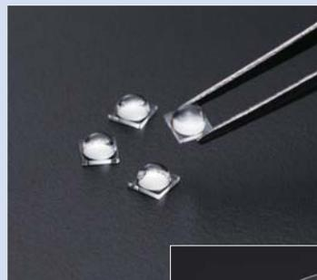
Micro-lenses for ultraviolet LEDs
