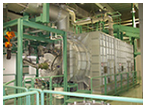
Rotary kiln combustible solid waste incinerator
